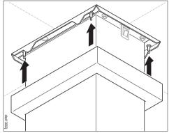
■ Finally, being careful not to scratch the chimney, push the cover plate upwards until the spring fixing clips click into place. If installed correctly, the cover should be secure and flush against the ceiling.
